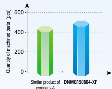
**Conclusion:** The insert proved to be superior to the similar products by A company in both efficiency and quality of the finished surface.
